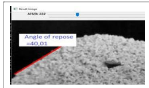
Figure 9c. AoR of granule A was measured at distance 17 cm
