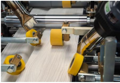
Fig. 2. Lamination process performed by the Soft Laminator (Profile Wrapping) machine.
