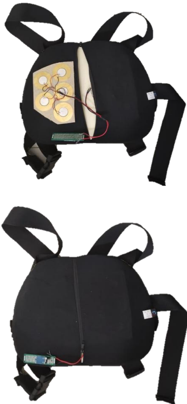
Fig.13. Simulation of piezoelectric installation on Piezo-Powered Ergo-Lumbar Support Device prototype (opened and closed)
