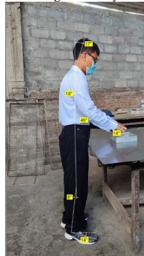
Improvement work posture of cutting the dough by machine
