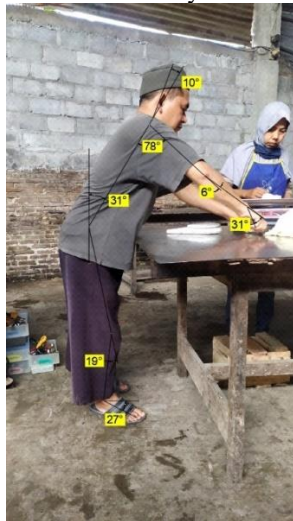
Initial work posture of cutting the dough by machine
